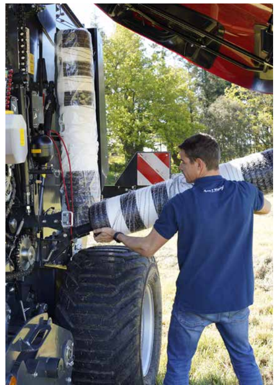
The smart net roll storage allows a comfortable horizontal loading.
