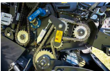
Rotor chain transmission with 1¼" pitch chains.
